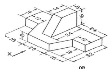
Q.5(B) Draw the isometric view of the object, the multi view projection of which 14M 5 3 is shown below:
