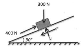
Q.6(A) A 50 kg block rests on a horizontal floor for which coefficient of friction is 0.3. If a block is subjected to a force of 400 N as shown in figure, find velocity of a block (in  $m/\sec^2$ ) after 3 sec. Assume, a = 10  $m/\sec^2$ .
