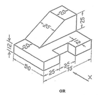
Q.5(B) Draw the isometric view of the object, the multi view projection of which is shown below:
