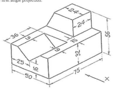
Q.5(B) Draw the isometric view of the object, the multi view projection of which 14M 5 3 is shown below:
