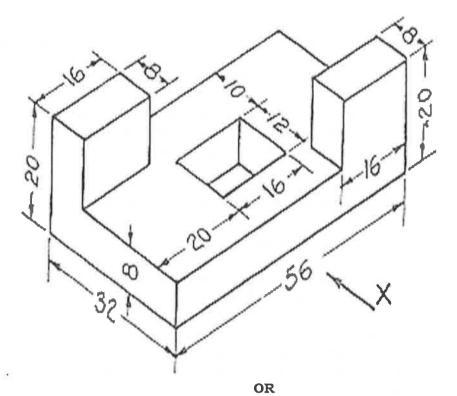
Q.5(B) Draw the isometric view of the object, the multi view projection of which 14M 5 is shown below:
