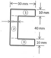
Q.4(B) Locate the Centroid of the Plane lamina as shown in figure.
