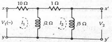
(ii) Find the equivalent star network from the circuit given below: 6M 3 3
