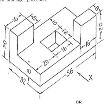
Q.5(B) Draw the isometric view of the object, the multi view projection of which 14M 5 is shown below.
