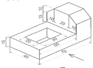
Q.5(B) Draw the isometric view of the object, the multi view projection of which is shown below:
