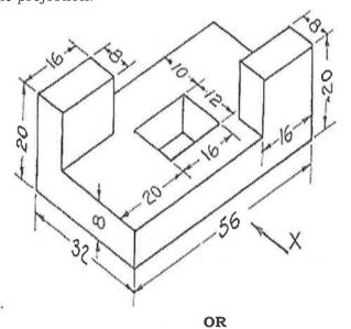
Q.5(B) Draw the isometric view of the object, the multi view projection of which 14M is shown below:
