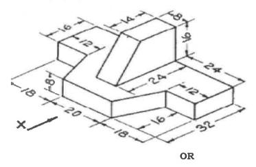
Q.5(B) Draw the isometric view of the object, the multi view projection of which 14M 5 is shown below.
